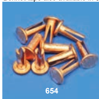
654 Copper split bifurcated rivet. 7.5mm head, stem 3.8mm x 11mm. For fixing bonnet tape etc. Sold in packets of 10 pieces.
