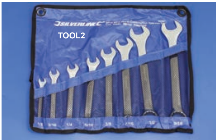
TOOL2 8 piece BSW Whitworth spanner set in holder pouch. Chrome finish spanners with open end at one end, ring spanner at the other. Drop forged, hardened and tempered. Chrome vanadium steel. Sizes 1/8", 3/16", 1/4", 5/16", 3/8", 7/16", 1/2", 9/16"
