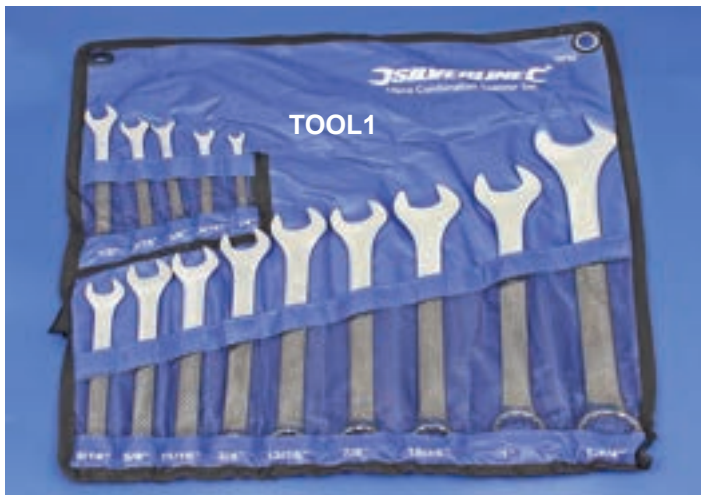
TOOL1 14 piece AF spanner set in holder pouch. Satin chrome finish spanners with open end at one end, ring spanner at the other. Drop forged, hardened and tempered. Chrome vanadium steel. Sizes 1/4", 5/16", 3/8", 7/16", 1/2", 9/16", 5/8", 11/16", 3/4", 13/16", 1" and 1.1/4".
