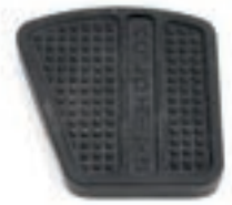
Special Pedal Rubber Ford SKU: HT100L Equivalent to original Holdtite pattern No.100. Handed. Internal recess for pedal vertical and top dimensions 2 3/8" x 2 3/8"
