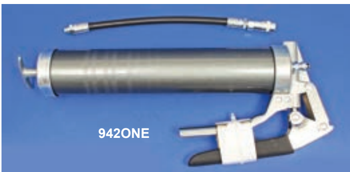
942ONE Professional one hand grease gun. one handed operation grease gun, complete with 9" flexible hose and four jaw hydraulic connector. For 400g cartridges or 500g bulk fill. Suitable for use with silicon grease. Max pressure 300 bar.
