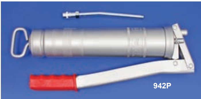
942 Side lever grease gun Top of the range side lever grease gun complete with 6" rigid, cranked extension tube and precision four jaw connector (for hydraulic nipples) - for 400g cartridges or 500g bulk fill. Short stroke delivery system - 1.5cc per stroke, max pressure 800 bar.
